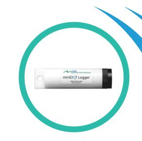
The miniDOT® Logger is a completely submersible instrument that logs dissolved oxygen and temperature measurements. The oxygen sensor is an optode that measures dissolved oxygen concentration in water through a fluorescence method. Data are recorded to an internal SD card. Operation of the miniDOT logger such as setting the time and sample interval can be accomplished via the USB cable.
